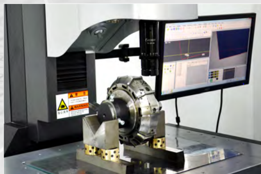
▲ 影像测量仪检测刀具 Image measuring instrument is detecting milling cutter
